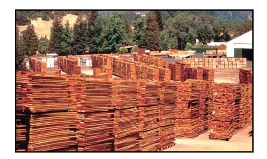
With over 200,000 square feet of covered storage, you can be assured of receiving bright stock on a timely basis. The Asti facility also includes a high-speed planer, an 8-bin tray sorter with resaw and an automatic sticking machine capable of processing 200,000 board feet per shift. Our computerized lathe, which is capable of handling 6x6 timbers up to ten feet in length, produces a variety of turned products such as spindles, balusters and balltops.
